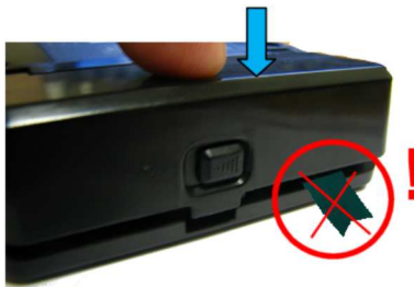
Figure 15: NR-1207-E / NR-1207-3 battery installation
