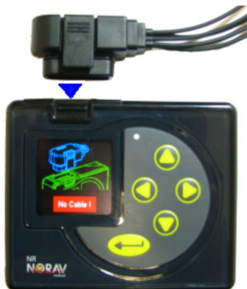
Figure 13: NR-1207-E / NR-1207-3 Patient Cable Connection
